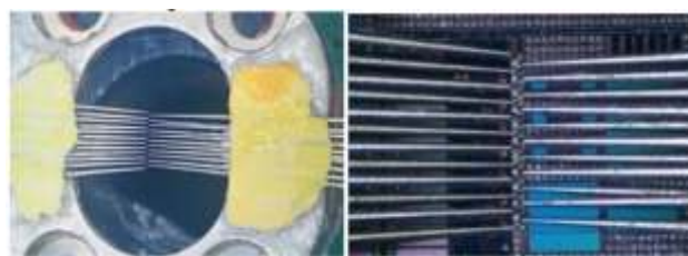
Figure 23: Two tier assembly of probe pins
