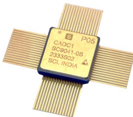
Figure 15: SC9041_0S in 64 Pin CQFP
